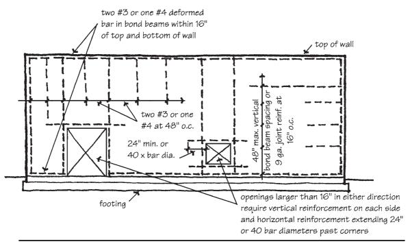
MASONRY ELEMENTS WHICH ARE NOT PART OF THE LATERAL-FORCE-RESISTING SYSTEM reinforcement required in either the vertical or horizontal direction
