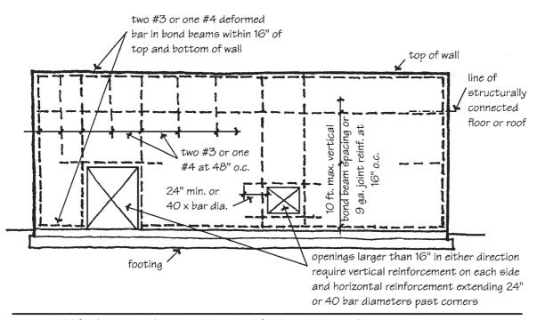
MASONRY ELEMENTS WHICH ARE PART OF THE LATERAL-FORCE-RESISTING SYSTEM reinforcement required in both the vertical or horizontal direction
